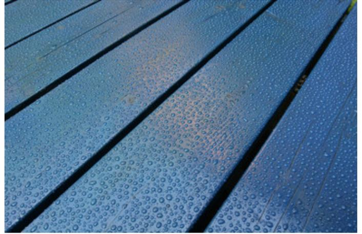
The correct priming and finishing of hard wood especially for exterior exposure is a complex matter and the wrong choice of product can result in premature break down in the paint system and subsequent deterioration in the wood. We are pleased to be able to supply a specially developed microporous system from Sirca which gives a minimum life expectancy of 5 years exterior exposure on correctly prepared and coated hard woods
